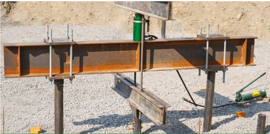
TENSION LOAD TEST
